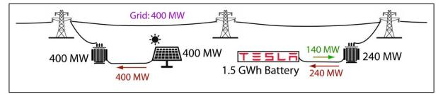
The full 400 MW from the solar array/inverters is sent to the grid via a 400 MVA transformer. The battery substation requires a 240 MVA transformer (max charge rate).
